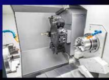
Main and Sub Spindle with Sauter BMT 65 Turret.
